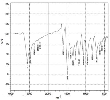
Fig. 2 FTIR-Raman Spectroscopy of 5-phenyl-1,3,4-oxadiazole-2-thiol
